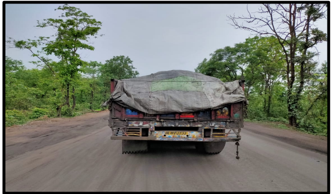
Covering coal trucks with tarpaulin sheets for Controlling dust.
