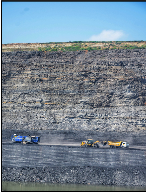
Production through surface miner and loading for dispatch at Lakhanpur and Bharatur OCP's
