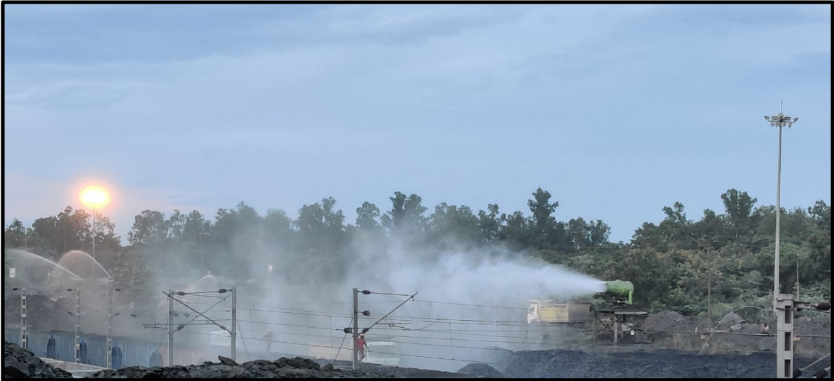
Trolley mounted Fog cannons (100m throw) at siding no.6, Lakhanpur OCP
